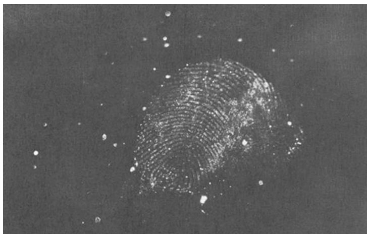
FIG. 2—Fingerprint developed on an apple with black powder tagged with coumarin 6 laser dye.
