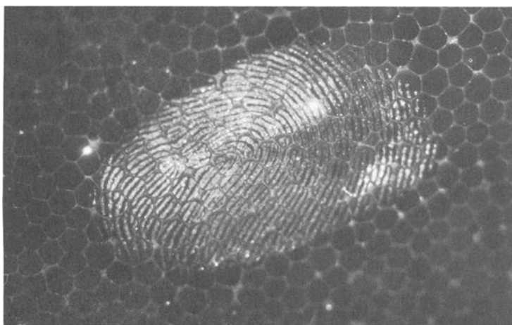
FIG. 1—Fingerprint developed on Styrofoam® cup with black powder tagged with coumarin 6 laser dye. The laser configuration and operation are as described by Dalrymple et al [1].
